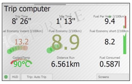
The screen gives you the key values on your current trip or other selected time interval, enabling evaluation of overall trip efficiency and cost, as well as instant consumption values. Most of the parameters are displayed for the currently selected time interval (current trip by default).
