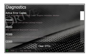
sure you don't need this information anymore as deleting the codes will remove the "Freeze Frame" data, which could be useful in diagnostics during car servicing.
