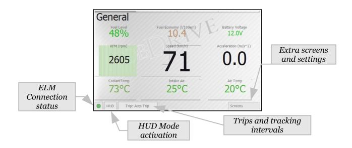
HobDrive is controlled by tapping the touch-screen elements and screen controls or by touching and scrolling (panning) the elements for browsing and accessing the information outside of the current screen.
