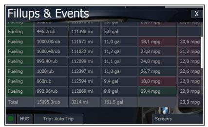
The screen is used for the analysis of information on filling stations and hobDrive-stored events.
