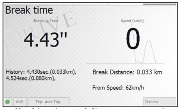
The measurement of braking time and distance at a certain speed. Helps to estimate the efficiency of the braking system, and to experiment with braking styles in dangerous road conditions.
