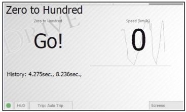
This screen used to measure vehicle efficiency in 0-100 km/h acceleration. The measurement starts automatically when you start driving. Depending on the refresh rate of movement sensors, the end result may not be entirely accurate.
